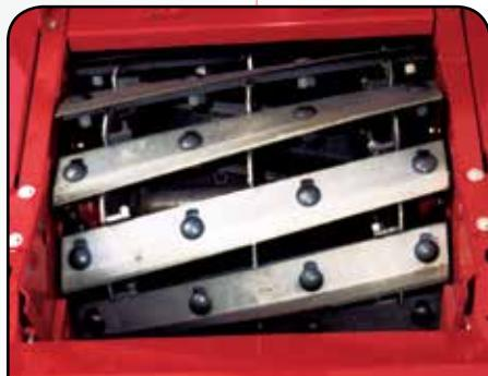
The **cutterhead** is a massive 24" (69 cm) wide by 22" (56 cm) diameter. This mammoth 450 lb (205 kg) cutterhead features full width, solid steel knife supports, to securely fasten the 12 full width, tungsten coated, helicoidal knives.
