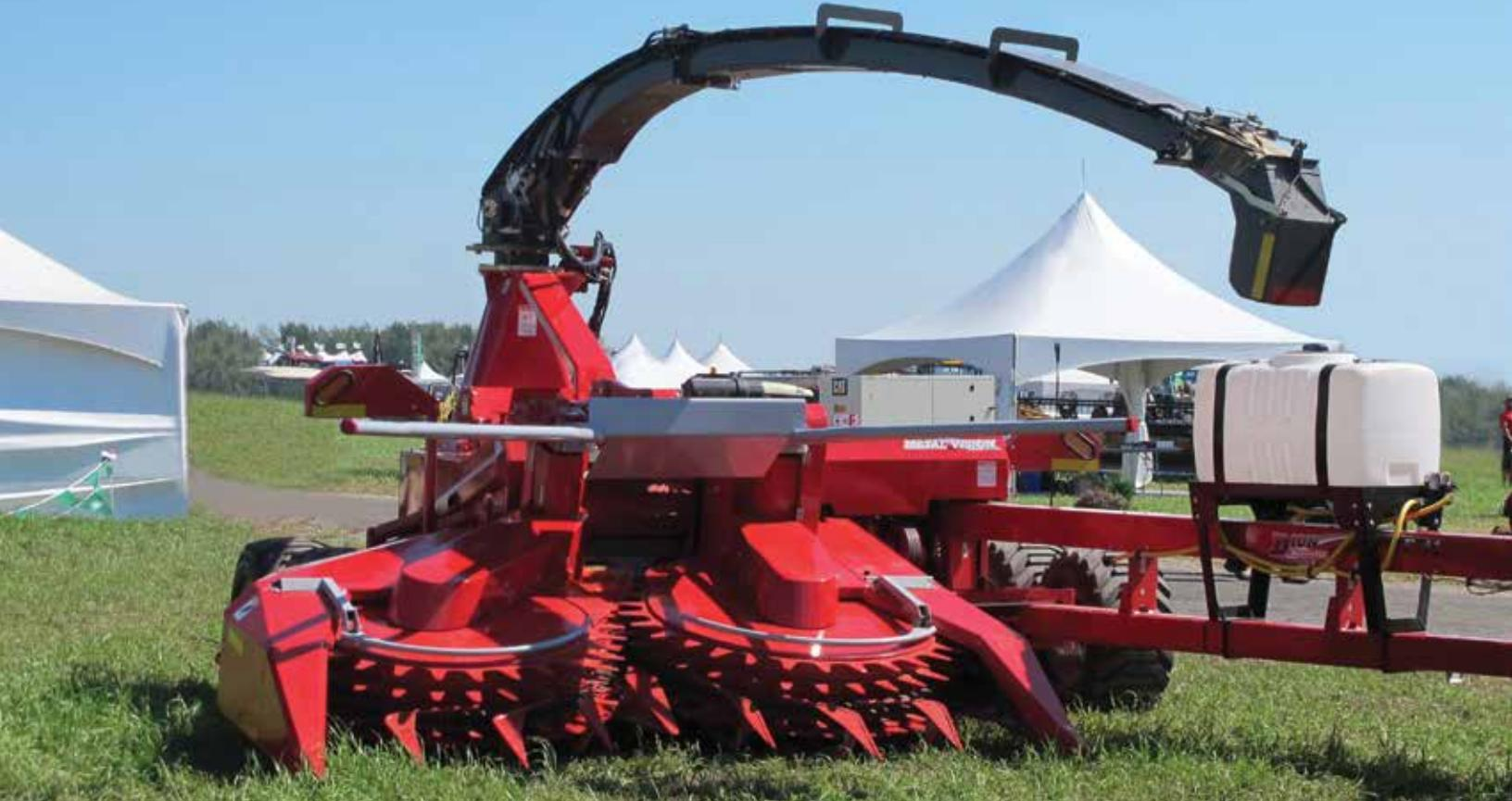
**Easily load to the left or right**, the stinger raises up to a height of 18.5' (5.6 m) with a length of 18' (5.5 m) and offers 280° rotation with a 4 m minimum reach. The modular design is convertible from the side loading to a trailed loading configuration.
