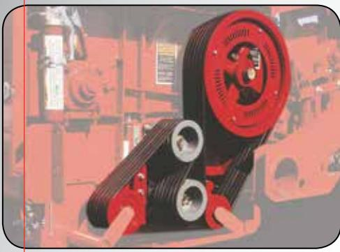
The **kernel processor** rolls are designed with height adjustment using a single wrench. The rolls are adjustable from a minimum clearance of  $1/16"$  (1.6 mm) to a maximum clearance of  $1.5"$  (38 mm).
