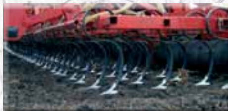
Equipped with spring tines and duck foot
