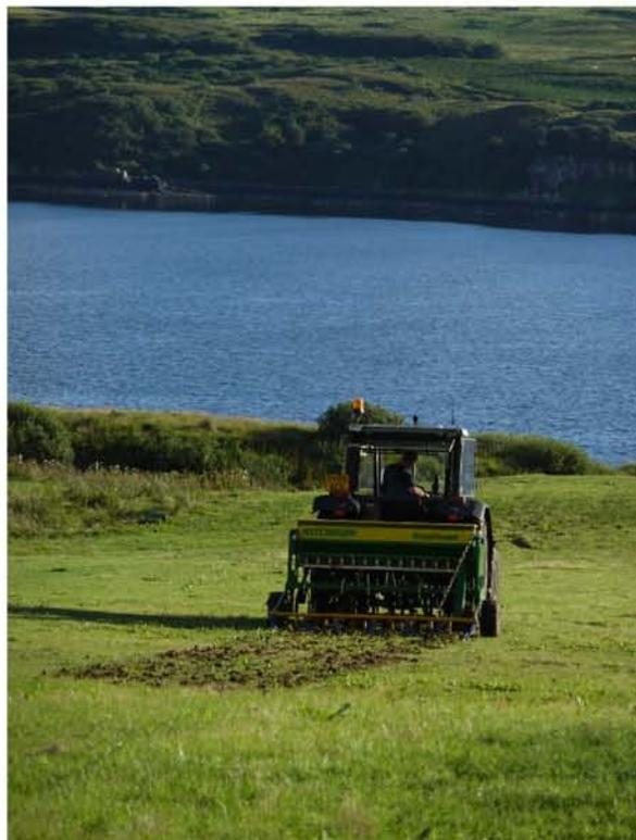
**AITCHISON** tine drills with their unique 'inverted T' boot were developed in New Zealand during the 1970's, providing a radical and effective solution for introducing new productive and appetising grasses and clovers into an existing sward with a minimum of expense and upheaval.
