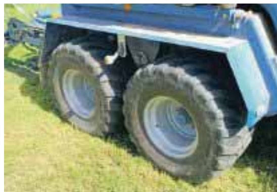
All the components are incorporated on a heavy duty tandem axle chassis that is supported on 500/50-17 tyres.
