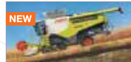
NEW AUTO SLOPE adjusts the fan speed to maintain the crop flow in the cleaning system no matter which angle the combine is working at.
